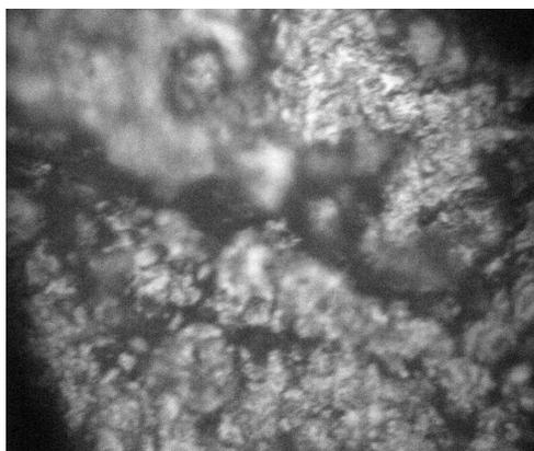
Fig. 1. Microphotography of surface of the hardened unmodified UFR-sample (KF-MT-15). X 300.
